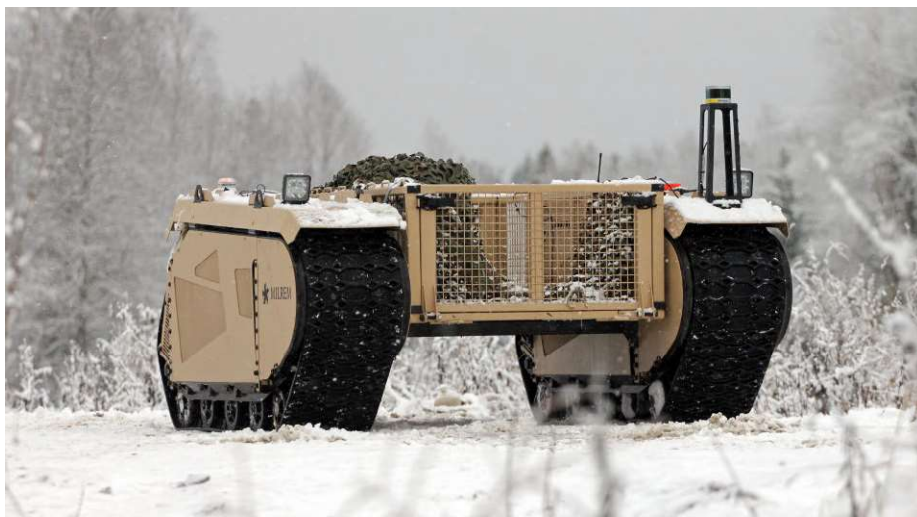
The Tracked Hybrid Modular Infantry System (THEMIS) is a hybrid fully modular unmanned ground vehicle. The Milrem Robotics vehicle is intended to provide support for dismounted troops by serving as a transport platform, remote weapon station, IED detection and disposal unit, and much more.
